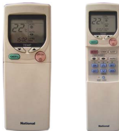
Gambar 5. Remote Control AC National (dengan Sliding Cover)
