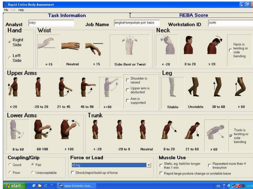
Figure 4. The REBA assessment of worker's body posture at sorting workbench
